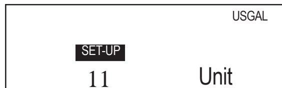
Fig. 5: Example of sub-function 11; unit for Total..
