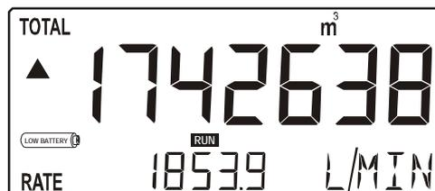
Fig. 4: Example of low-battery alarm.
