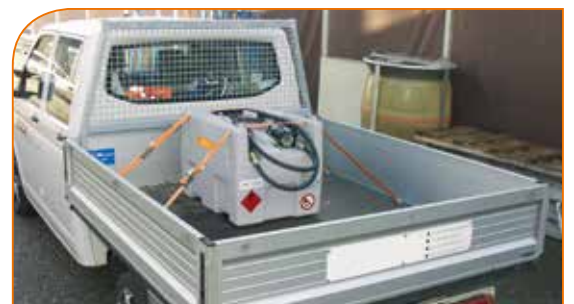
Recesses for ratchet lashing strap
